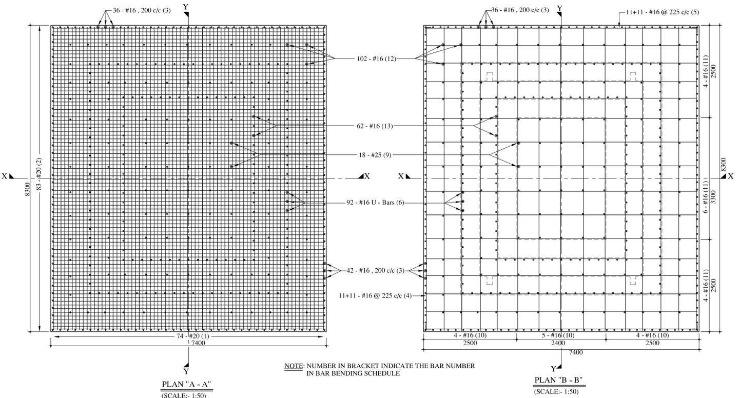
NOTE: NUMBER IN BRACKET INDICATE THE BAR NUMBER IN BAR BENDING SCHEDULE
